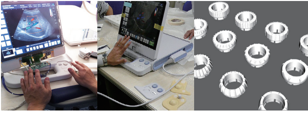
Fig. 11 In developing the UI (user interface) design, feedback from doctors and sonographers was repeatedly incorporated in a series of ever-improving UI designs.
