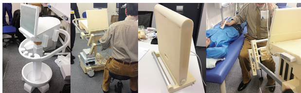
Fig. 1 In the early stage of designing the SONIMAGE HS1, we verified the performance of its functions and operation design using rapid prototyping.
